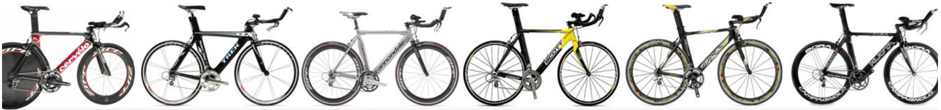
Pre DA: TT bike structures are with simple, straight tubular forms, some have partial wheel cut-outs
