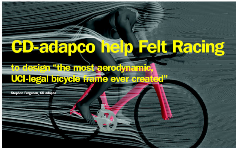
Fig.01 The Felt DA is the fastest UCI legal Tri / TT bike built today. Developed over two years with careful use of NACA airfoil profiles, CFD flow modelling and wind tunnel experimentation, the DA frame system delivers unsurpassed aerodynamic advantage with incredible time-trial and steering stiffness.
