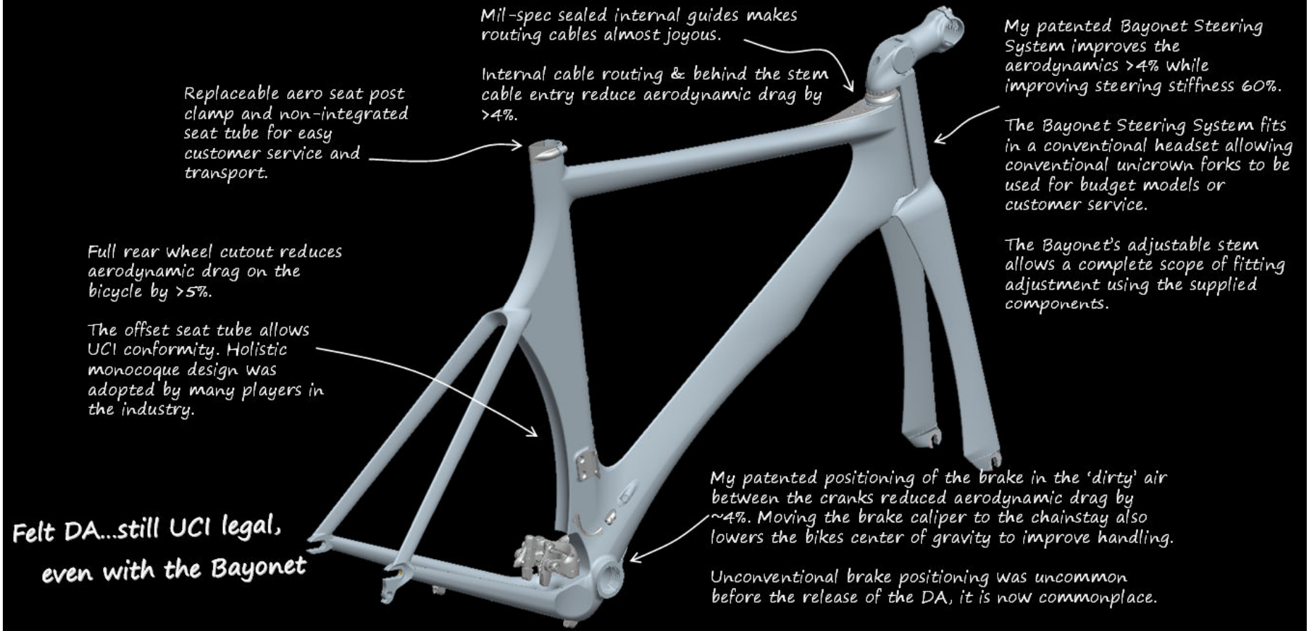
Post DA: integrated brakes, novel steering systems, elongated airfoil monocoque forms are commonplace
