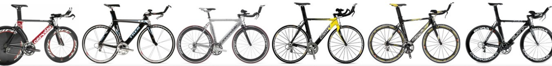
Pre DA: TT bike structures are with simple, straight tubular forms, some have partial wheel cut-outs
