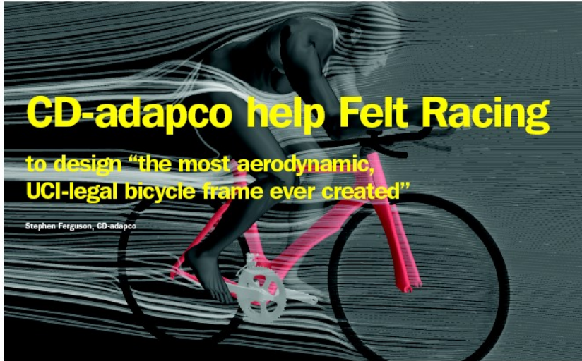
Fig.01 The Felt DA is the fastest UCI legal Tri / Tri bike built today. Developed over two years with careful use of NACA airfoil profiles, CFD flow modelling and wind tunnel experimentation, the DA frame system delivers unsurpassed aerodynamic advantage with incredible time-trials and steering stiffness.
